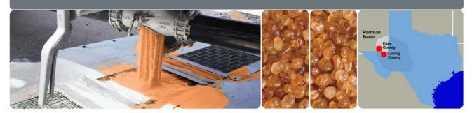
OilPlus<sup>™</sup> proppants are specifically designed for fracturing treatments in oil and liquids-rich reservoirs. These advanced proppants continue to outperform offset wells in many major basins throughout North America. They are field proven in over 1,000 wells with one billion pounds pumped so far.
