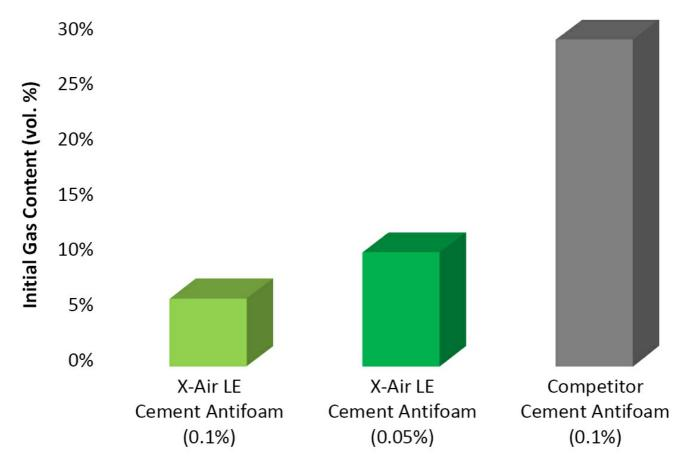
The X-Air LE liquid cement antifoam is more than five times as effective as the competitor at 0.1%. Even at half the concentration, X-Air LE cement antifoam is still over two and a half times as effective as the competitor.
